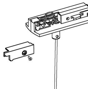
3. Pull the wire upwards to the needed length, cut off excess wire, then connect L, N, ground wire in right position again.
