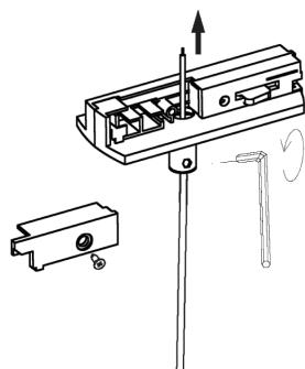
4. The screw needs to be locked after the adjustment is completed.
