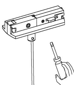
2. Unscrew these 3 screws, take out the L, N and ground wire.
