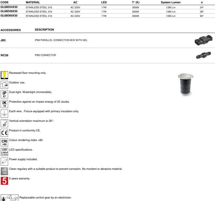
Replaceable LED light source by an electrician. (r))))()
