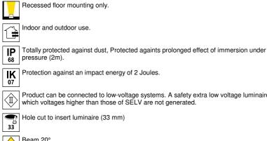
Product can be connected to low-voltage systems. A safety extra low voltage luminaire in which voltages higher than those of SELV are not generated. Hole cut to insert luminaire (33 mm)
